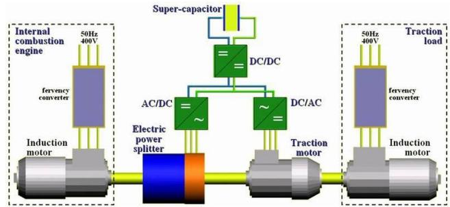
Fig. 3 Laboratory experimental working stand of HEV-CVUT
