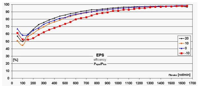
Fig. 6 Experimental characteristics of EPS efficiency
