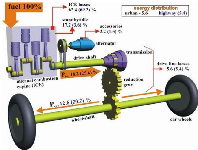
Fig. 1 Energy flow (from fuel energy to the wheels) for a midsize automobile
