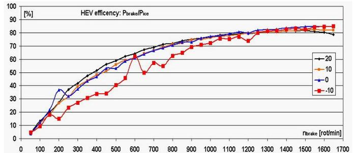
Fig. 5 Experimental characteristics of HEV system efficiency
