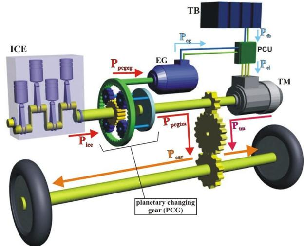
Fig. 2 Configuration of Toyota's parallel/series drive (THS drive)
