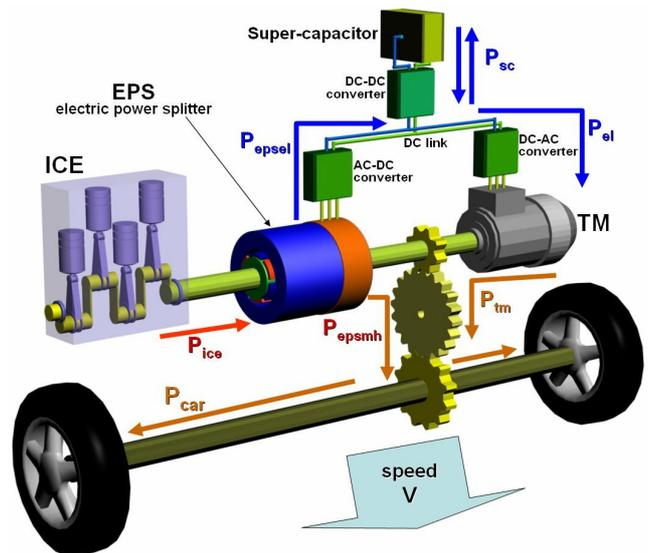
Fig. 3 Configuration of HEV-CVUT concept of HEV drive
