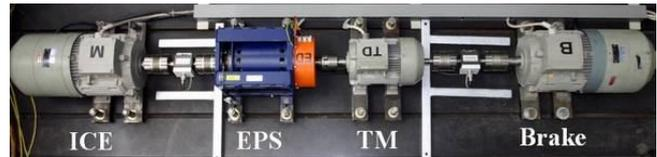
Fig. 4 Electrical machines of the laboratory working stand
