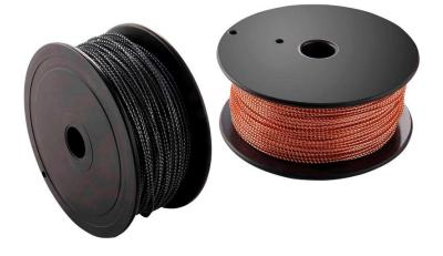
The Acme **Sealing Wire** is available in galvanized steel, copper and stainless steel and can be supplied on plastic spools or in cut lengths. The wire consists of a centre core wire and an outer wire, which is spirally lashed around the inner core wire providing an excellent thread type grip to prevent slippage or removal after the seal has been compressed.
