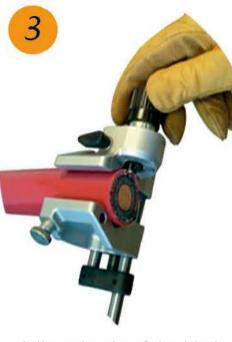
Adjust the tip of the blade up to ≈ 0.5mm from the screen
