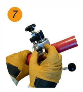
Put the blade lever in position "OFF" corresponding to the straight cut
