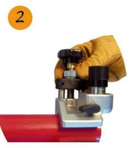
Lock the adjustement using the locking nut
