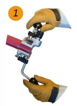
Put the tool on the cable without free but with possiblity to turn
