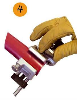
Put the black lever at the position "ON" corresponding to hélicoïdal cutting
