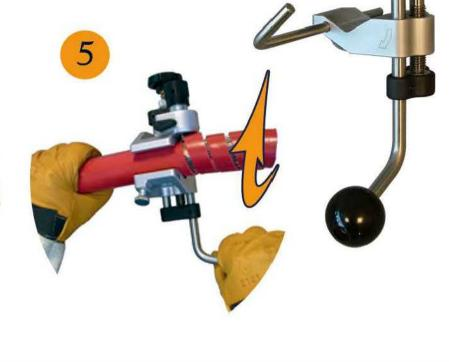
Strip the sheath, turning the tool clockwise with the handle
