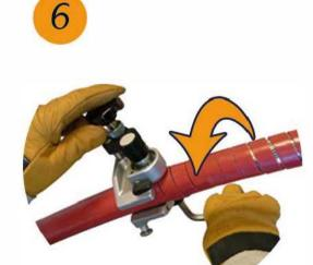
Arriving the stripping limit (note the width of the tool is 50mm), stop the tool, and Office Bitola: +389 (0) 47 20 to back half a turn
