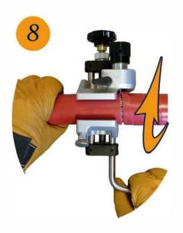
Finish with the straight cut turning 2 turns
