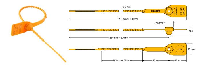
The Acme **Griptight Seal** is a heavy duty pull-tight seal manufactured from two dissimilar materials. The acetyl insert is durable and will withstand freezing and boiling conditions, whilst the nylon body is flexible for easy use. The design features rolled heat staking technology to secure the insert to the body, which provides clear evidence of tampering if forced open or cut. This seal is suitable for most applications where strength is a requirement.
