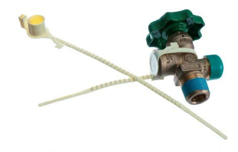
Our **Valve Seals** are special purpose variable length seals designed for use on Oil and LPG gas cylinders or valves. Manufactured in polypropylene material the seals are very flexible and can be applied easily by hand. The design includes a simple tear off tag for removal without tools.
