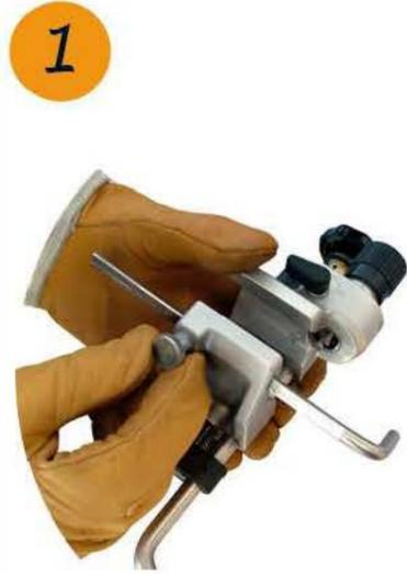
1 Introduce the graduated gauge and lock at the needed position
