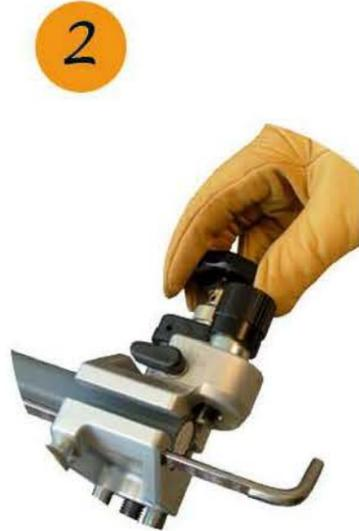
2 Put the tool on the cable without free but with possibility to turn
