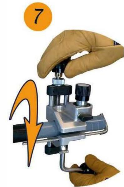
7 When you arrive at the stripping limit (end of the graduated gauge in contact with the core), stop the tool and turn back half a turn
