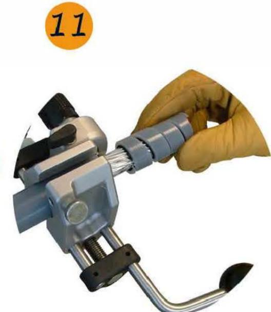
11 Remove the insulation and the tool
