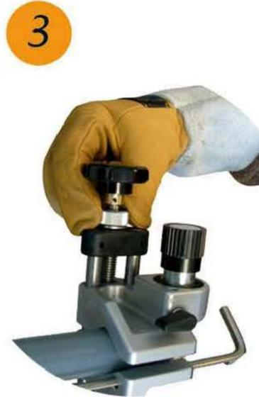
3 Lock the adjustment using the locking nut
