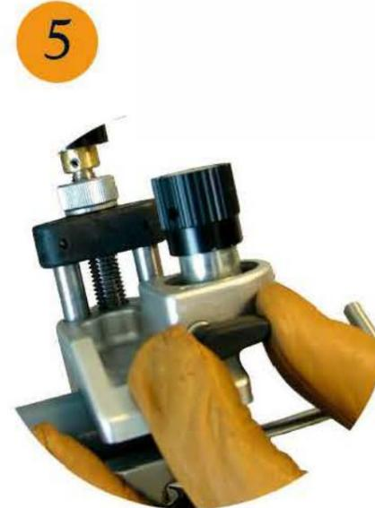
5 Put the blade lever at position "ON" corresponding to the hélicoïdal cutting
