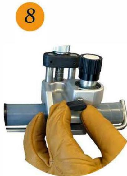
8 Put the blade lever in position "OFF" corresponding to the straight cutting
