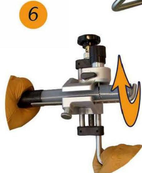
6 Strip the insulation turning the tool clockwise with the handle
