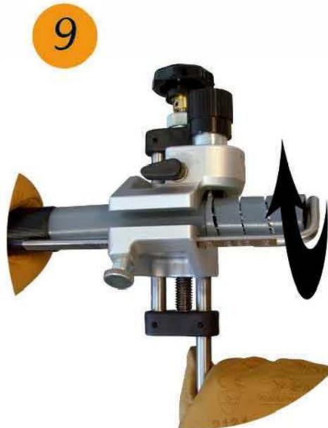
9 Finish with the straight cut turning 2 turns
