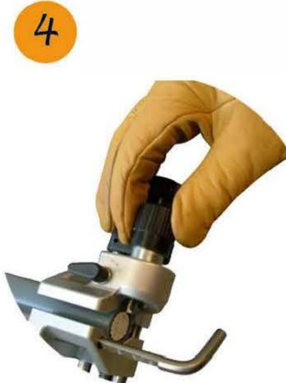
4 Adjust the tip of the blade up to ~ 0.5 mm from the cable core
